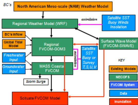
**Figure 1** Schematic of NECOFS, showing the three core models (WRF, FVCOM 3.1, SWAVE). Note that the Scituate FVCOM inundation forecast model system can be driven by either FVCOM-GOM3 or MASS Coastal FVCOM.
