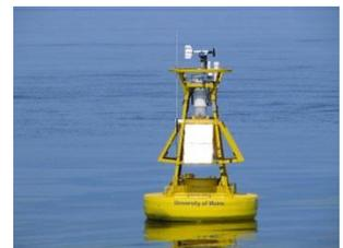
The University of New Hampshire (UNH) - Pacific Marine Environmental Lab (PMEL) buoy for monitoring of acidification and CO2 is now delivering data to NERACOOS.org. This system measures physical, chemical and biological data at the surface. These data are being used to unravel the relative contributions of atmospheric carbon dioxide, biological processes and freshwater dynamics to the ocean acidification issue. The data can be seen on the [NERACOOS site](#) and also on
